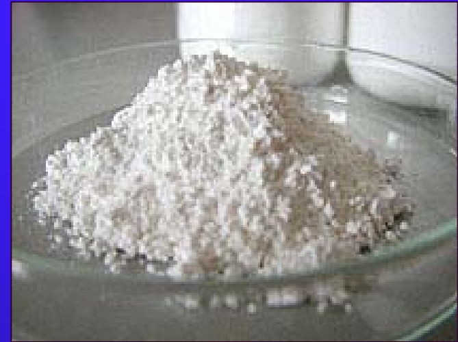
Hydrated lime – Dry Slaking
